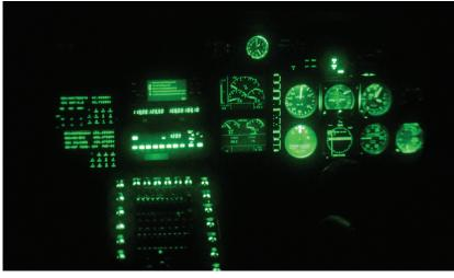
TOP NVIS-Class-B-modified cockpit lighting as viewed through Class-A objective lens ANVIS-9 NVGs. Making sure the NVGs and the rest of the NVIS are compatible is critical. In this instance, the unfiltered light being emitted in the 625- to 665-nanometer range will activate the automatic-gain-control in newer goggles, causing an ongoing loss of visual acuity for the scene outside the cockpit.
